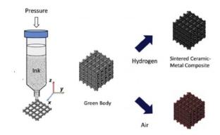
Sintering of micro-trusses created by extrusion-3D-printing of lunar regolith inks
