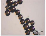
Glass fibers and hollow glass microspheres produced by melting the simulant at 1450°C in air
